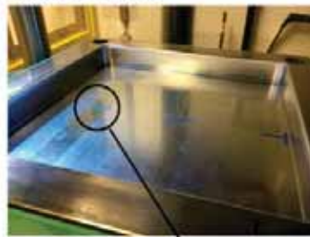
Preheating of tooling to defined curing temperature at 140 °C:
